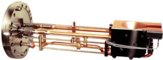
EV 1-8 UHV horizontally mounted on CF100 without cover
